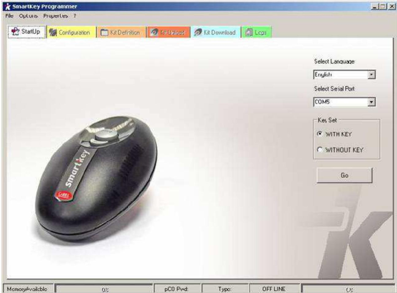
This is the first panel displayed by the program, and is used to set the port for communication between the program and the SmartKey, to select the language so as to better understand the messages shown in the program, and to set the program for operation with or without the key inserted.
