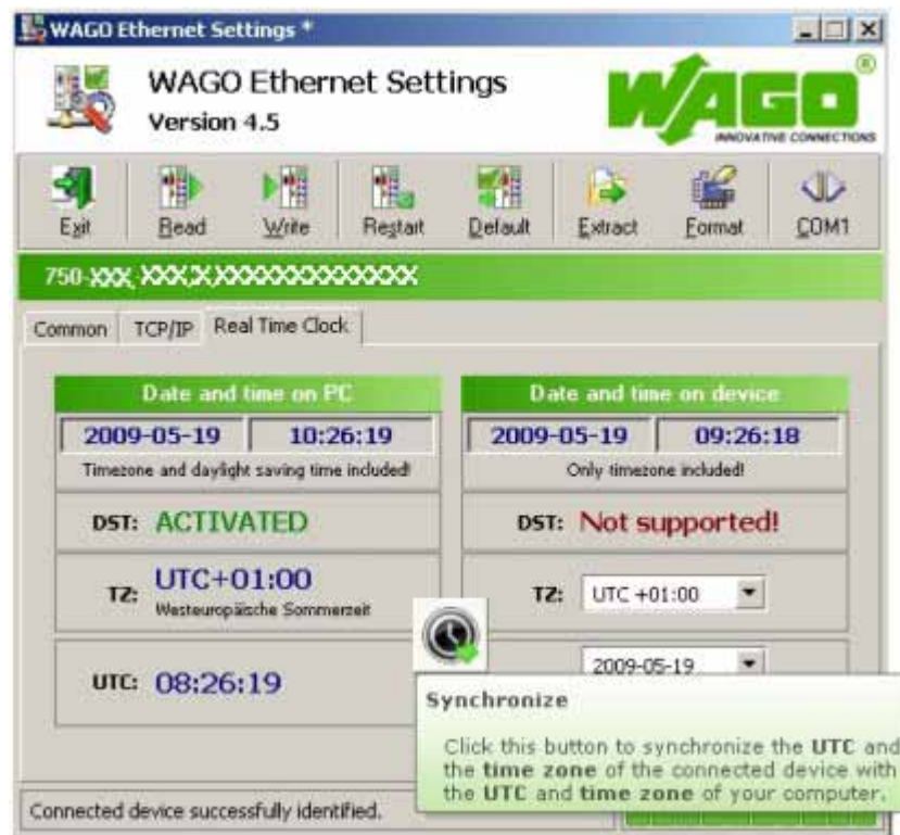
Figure 50: Example of real-time clock synchronization in ETHERNET Settings
